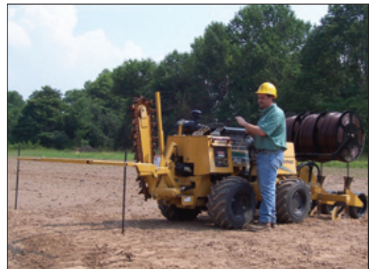
Figure 35 - Vermeer® LM42 shown with 3-blade vibratory plow. Standard tubing rack not shown on picture at right.
