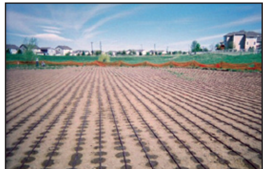
Figure 30 - Examples of wetted pattern of Techline CV after running for four minutes and prior to being covered with topsoil.
