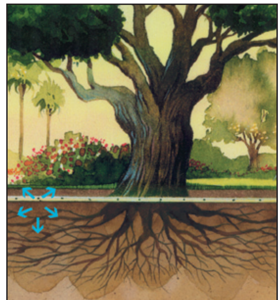
Figure 13 - The upward, outward and downward movement of water in a dripperline system.
