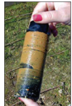
Figure 36 - The rings of this filter show how much dirt and debris can exist even in potable water, which this system is used on.
